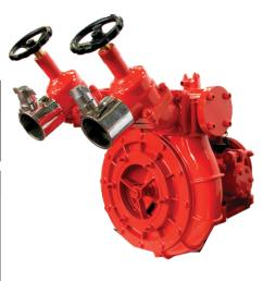
N K Fire® Multipressure Fire Pumps are designed for high performance and reliability. N K Fire® offers pumps of modern design suitable for Fire Brigade Services, Petroleum and Oil Gas Sectors and other Industries. N K Fire® manufactures Pumps with Discharge Capacities upto 6,000 LPM on Low Pressure and 400 LPM on High Pressure Side
